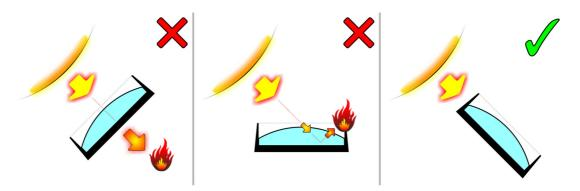
Figure 1. Avoiding damage from light sources
