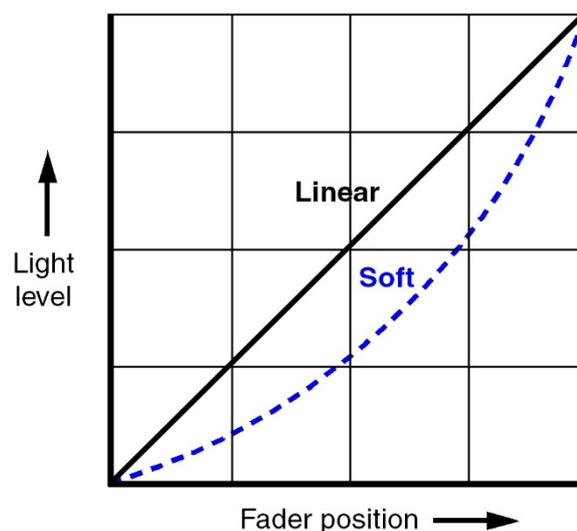
**Figure 1. Dimming curves**
