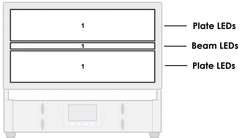
**Figure 3: LEDs grouped into Beam and Plate**
