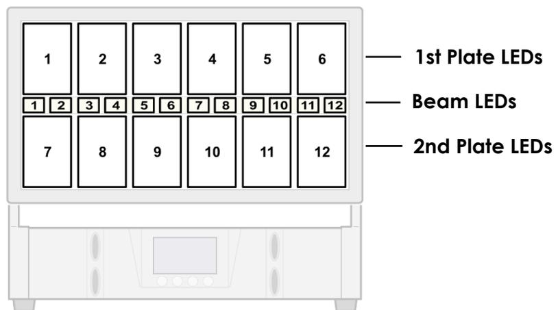
*Pixels are numbered as seen when looking at the front of the fixture with Tilt set to 000.*
