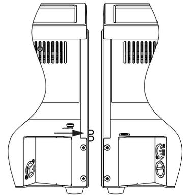
**Figure 9: Alignment pins**
