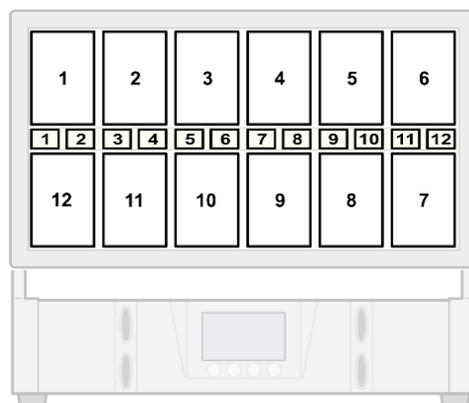
**Figure 6. Pixel orientation = OFF (Normal), 2<sup>nd</sup> Plate pixel orientation = ON (Inverted)**
