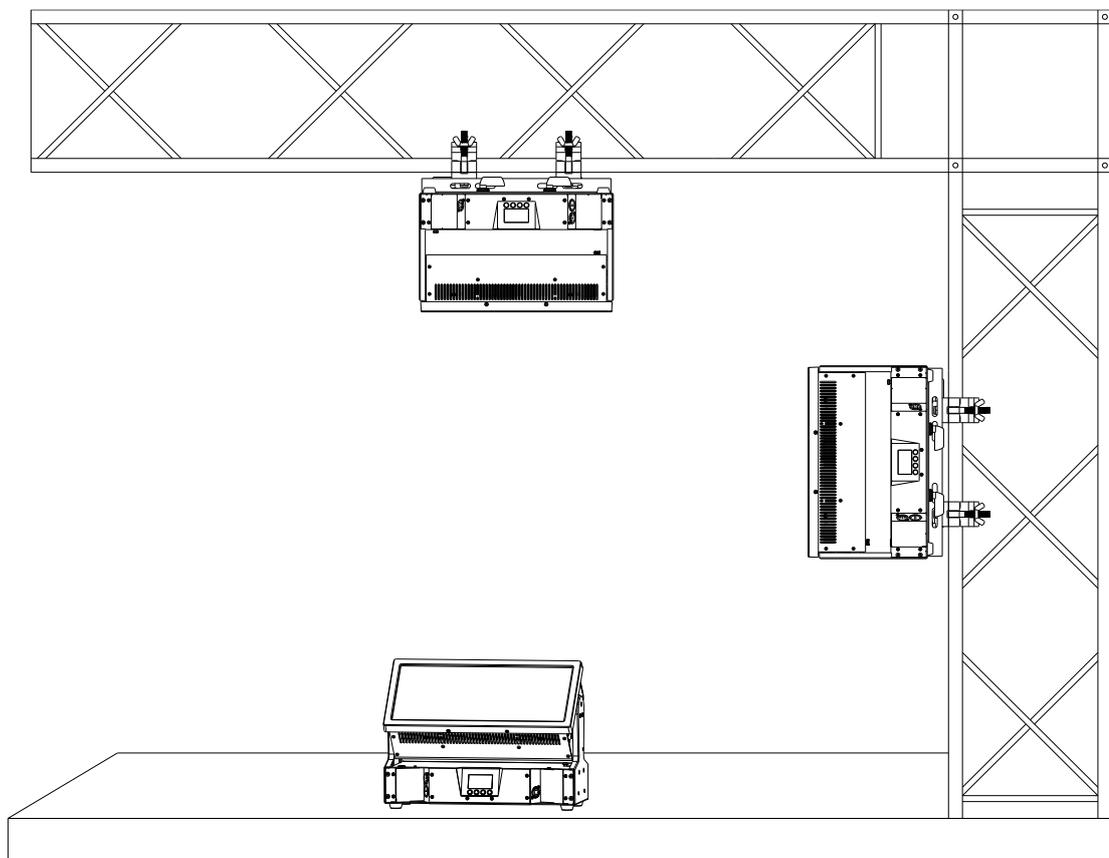
**Figure 8: Mounting options (safety cable not shown)**
