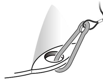
**Figure 6. Safety cable attachment**
