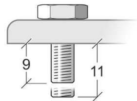
**Figure 4. Bolt protrusion**
