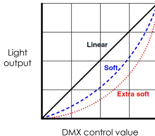
**Figure 3. Dimming curves**
