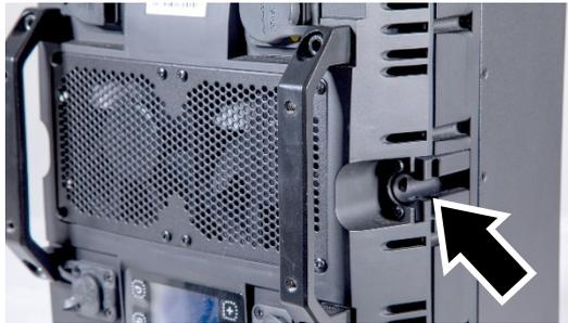
**Figure 5. Mechanical connector channel**
