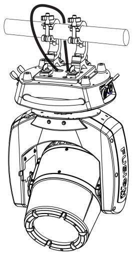
To secure an EXO Beam 10 fixture with a safety cable:
