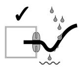
cable slack and create 'drip loops' before connectors.
