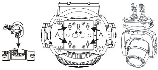
Figure 4. Omega bracket fasteners
