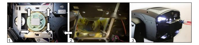
Figure 20: Lamp adjustment
