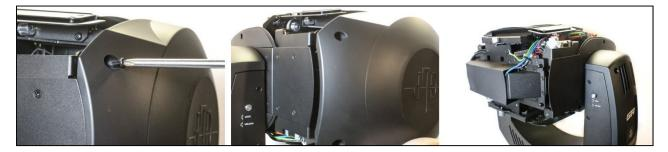
Figure 14. Rear head cover removal
