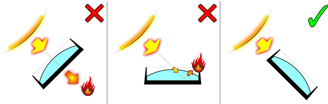
**Figure 1. Avoiding damage from light sources**
