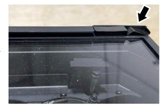
Figure 7. Front cover retaining clip
