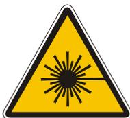
**Attention:** Laser Class 4 can cause injuries of your eyes even without optical instruments in front of them or within a distance of less than 1.5m and short exposure time.
