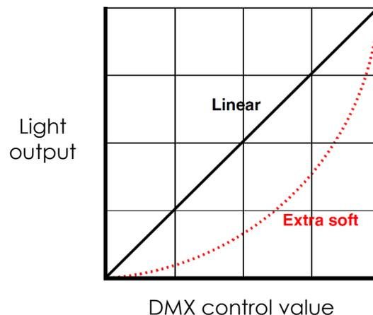
**Figure 7. Dimming curves**
