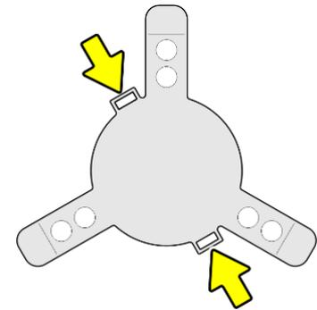
**Figure 11. Strap attachment points in tripod stand**
