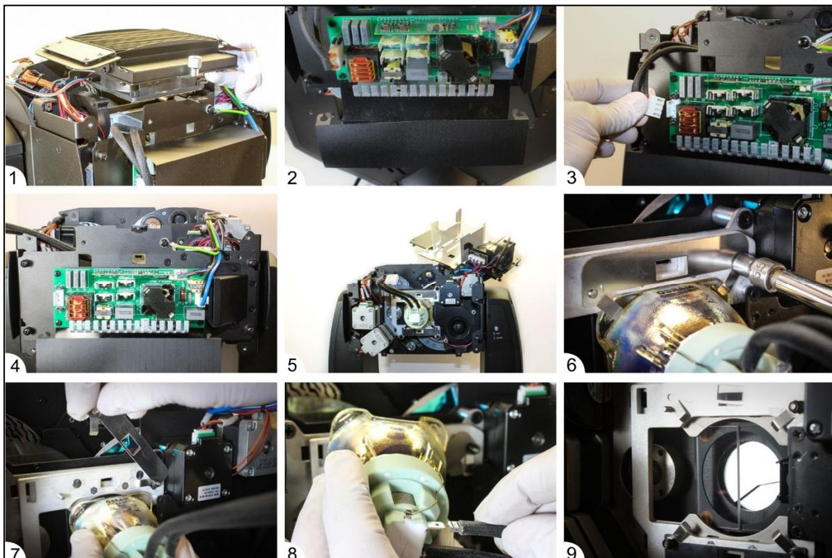
**Figure 18. Lamp removal**
