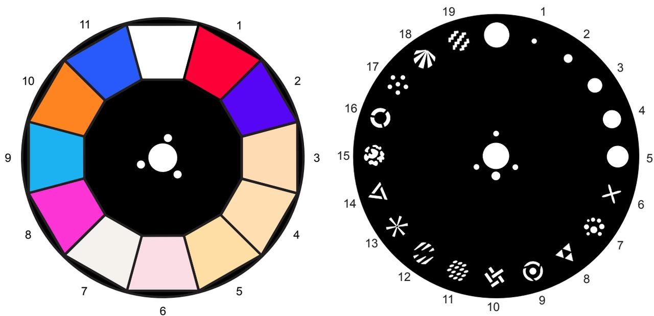
Figure 2. Color wheel and fixed gobo wheel
