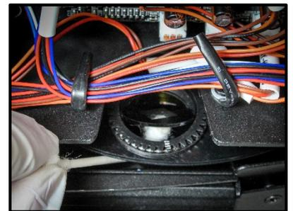
**Figure 15. Removing a glass gobo**
