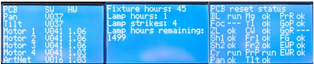
**Figure 12: Example of boot sequence and reset displays**
