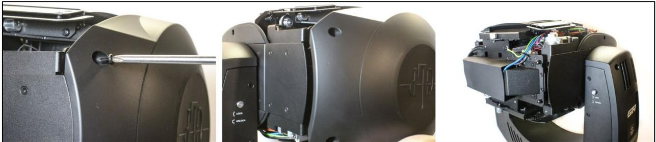
**Figure 14. Rear head cover removal**
