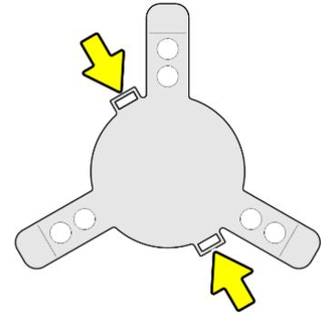
**Figure 8. Strap attachment points in tripod stand**
