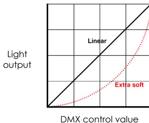
**Figure 4. Dimming curves**
