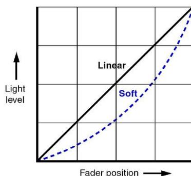
**Figure 2. Dimming curves**
